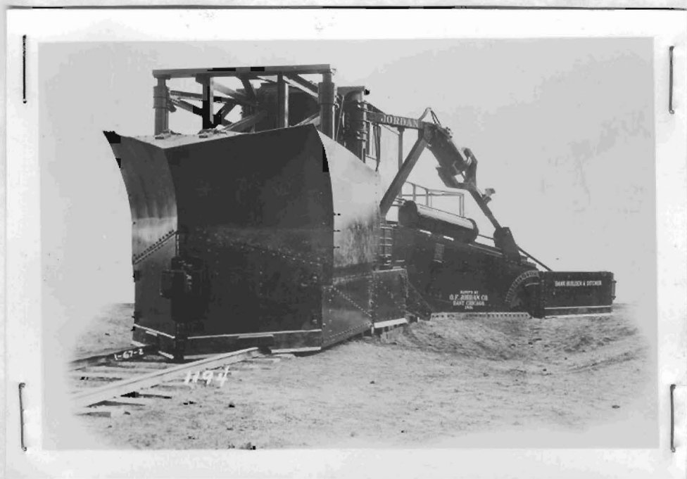
Three-quarter front view of a Type A JORDAN with high detachable Snow Plow. The plow in this picture is set to cut 3" below top of rail. The left wing is open in spreading form.
